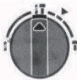
drilling with impact
